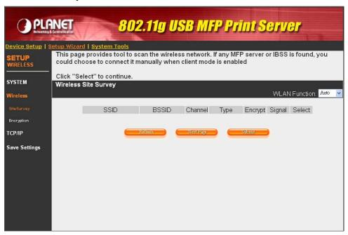
You can use this "Site Survey" function to search for available access points in you location. In the list is the information of all available access points or wireless stations includes SSID, BSSID, Channel, Type, Encryption and Signal Strength. You can select one wireless device in the list for this print server to associate with or you have to use General Setting to manually setup the wireless parameters.
